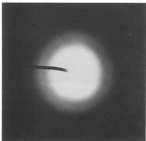
Figure 1 Electron diffraction pattern of as-prepared barium hexa-aluminate gel.
